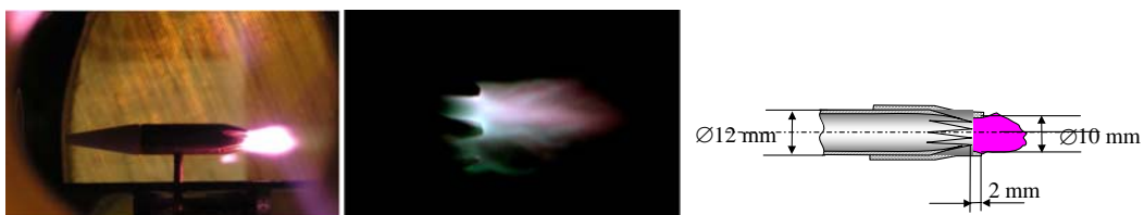
Figure 2. MW discharge initiated by passive vibrator with many sharpened tips in SS flow: general view, open lens – left, aft area, short exposition – middle, vibrator aft scheme – right.
