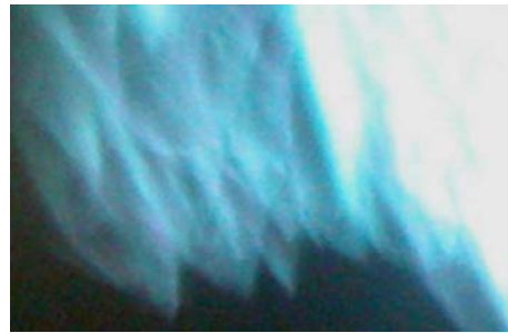
Figure 12. MW undercritical discharge fragment in supersonic flow of stoichiometric propane-air mixture ( \lambda = 2.5 cm; \tau_{pul} = 34 \mu s; v_{fl} = 5 \cdot 10^2 m/s)
