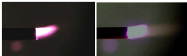
Figure 21. Deeply undercritical MW discharge initiated by a pipe-type EM vibrator in a supersonic air flow (left photo) and in a supersonic air with water aerosol flow (right photo) ( \lambda = 12.3 cm; E_0 \approx 10^2 V/cm \approx 10^{-2} \cdot E_{cr} )
