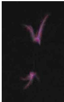
Figure.6. Deeply undercritical MW discharge initiated by EM vibrator with a diameter of 1 mm and length 7 mm ( \lambda = 2.5 cm; \tau_{pul} = 5 \mu s; E_0 = 0.1 \cdot E_{cr} ; p = 760 Torr)
