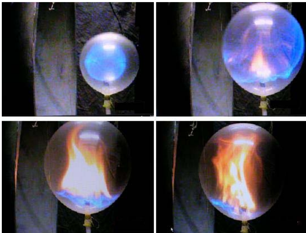
Figure 7. Sequence of frames from video-film in case of burning initiated by attached MW discharge (from the left to the right and from the top downward through 1/16 s)
