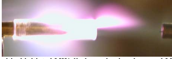
Figure 12. Deeply subcritical initiated MW discharge in air submerged MW stream at comparably high flow velocity
