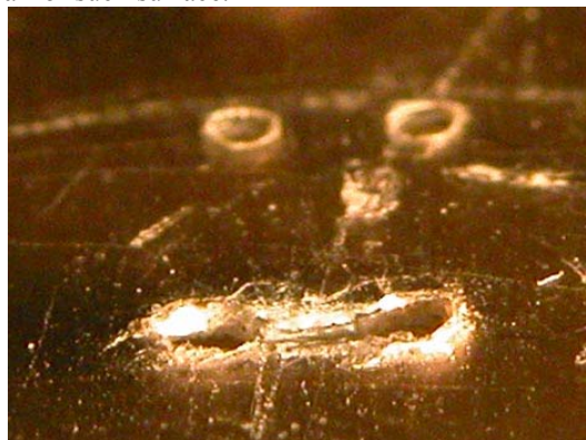
Figure 15. A surface of a sample of mica after 20 discharge cycles in the flow
