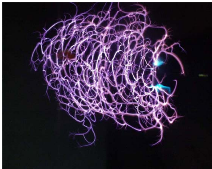
Figure 1. The typical view of subcritical streamer MW discharge.
