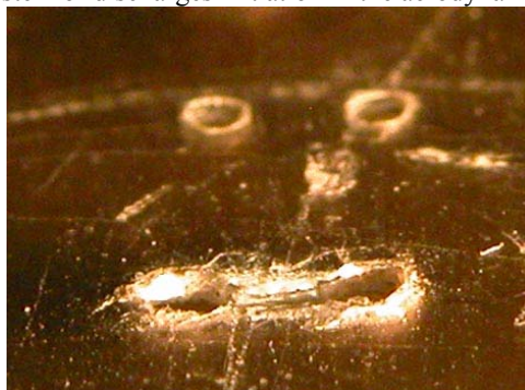
Figure 9. Mica sample surface after 20 discharge cycles in the flow
