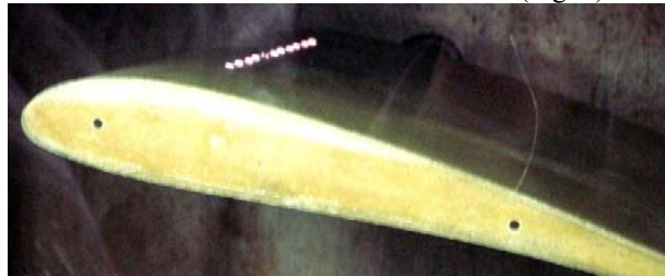
Figure 14. Wing model in a flow under an angle of attack with stable MW discharges over its surface, \lambda_z = 10\text{ mm}
